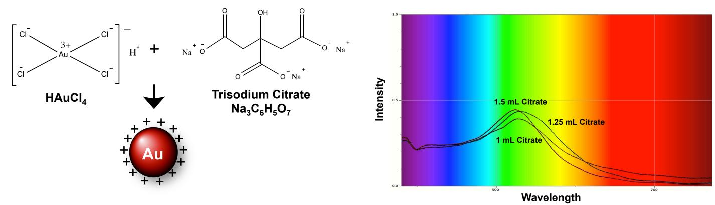
Increasing concentrations of Trisodium Citrate Dihydrate resulted in decreasing diameters of AuNPs and vice versa.
