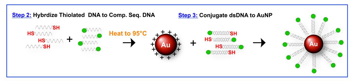
Both methods hybridize DNA via simulated Polymerase Chain Reaction (PCR) and attach DNAs to AuNPs using Au-S bonds, they differ only in the order in which these are done. Method 1 conjugates DNAs to AuNPs first, and hybridizes DNAs second. Method 2 hybridizes DNAs first, and attaches hybridized DNAs to AuNPs second.
