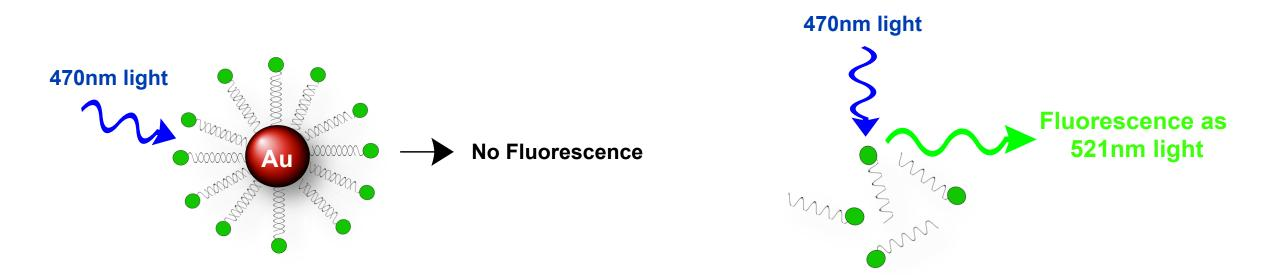
In intact DNA-AuNPs, electron transfer between FAM and AuNP causes quenching of FAM's fluorescence. Heating DNA-AuNPs dehybridizes dsDNA, releasing FAM-DNA. Upon thermal release, electron transfer between FAM and AuNP ceases and fluorescent functions return to FAM, enabling visualization of FAM-DNA.
