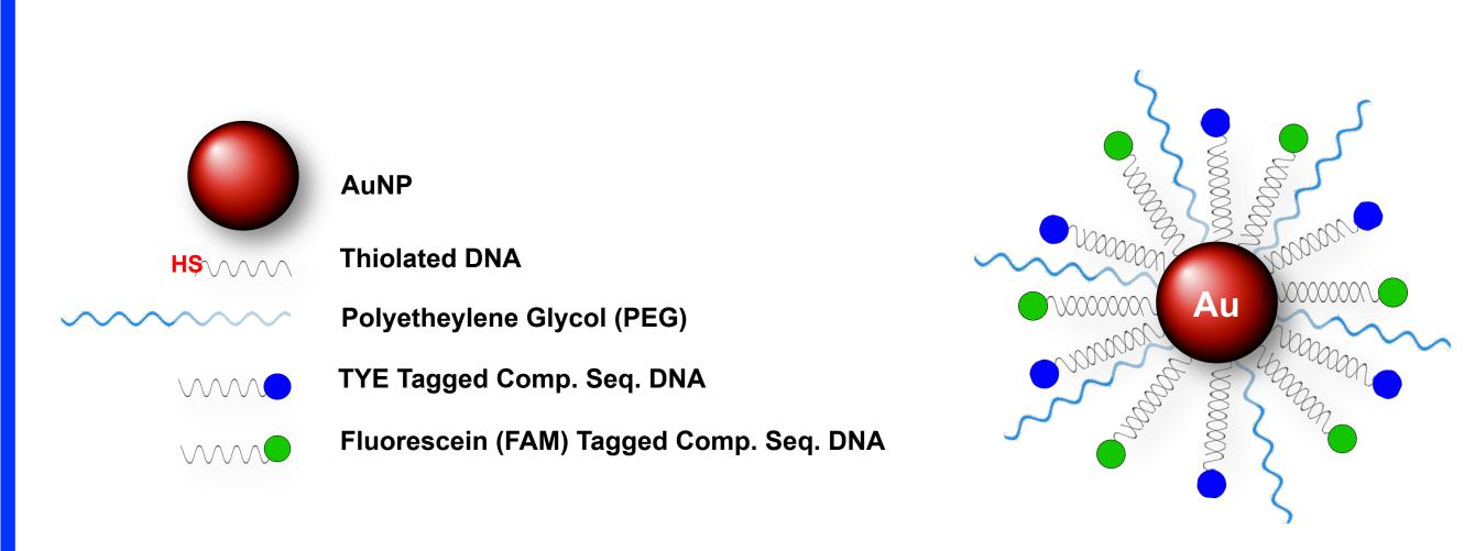
The drug delivery system seeks to eliminate some of the more prevalent side effects of chemotherapy by using a conjugated AuNP system. It is composed of a 20nm AuNP, Poly-ethyleneglycol (PEG), two different sequences of thiolated DNA, and two complimentary DNA sequences; one tagged with Fluorescein, the other with TYE.
