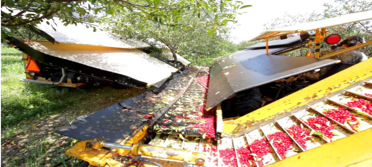
Figure 5.1. A standard cherry shaker. As you can see, the belt leads from the tree, across the belt and makes a 90 degree angle up towards bins of water. (Louis Gelder & Sons Co., 2015)
