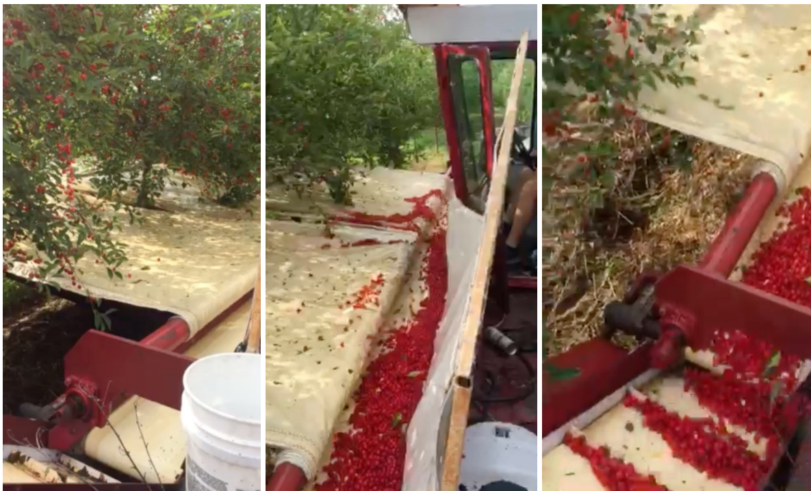
Figure 5.2. Steve's shaker. The tarp fits right to the tree root. The cherries fall onto the belt below and go directly over to the water bin, no 90 degree angles. Photos courtesy of the Grants.
